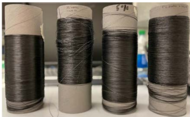
Figure 2: Nylon 6,6 fiber strands containing (10%, 3%, 5% and 8%wt respectively) graphene loadings.
