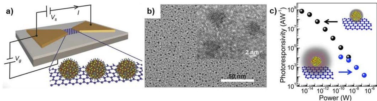
**Figure 1:** (a) Schematic diagram of the device and circuit arrangement. (b) TEM and high resolution TEM (inset) images of QDs (QD<sub>p500</sub>) deposited on a graphene oxide TEM support film. (c) Photoresponsivity versus incident power for QD<sub>TGL</sub>/SLG (black) and QD<sub>p500</sub>/SLG (blue) devices under  $\lambda_{ex} = 514$  nm illumination. Figure reproduced with permission from Ref. [10].
