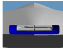
group 7 : outer part of exhaust duct T_{avg,7} = 295 \text{ K} \epsilon_7 = 0,92 Lambertian
