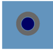
group 6 : Disc exhaust entry T_{avg,6} = 627 \text{ K} \epsilon_6 = 0,99 Lambertian
