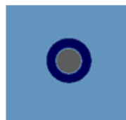
group 3 : Disc bypass entry T_{avg,3} = 295 \text{ K} \epsilon_3 = 0,9 Lambertian
