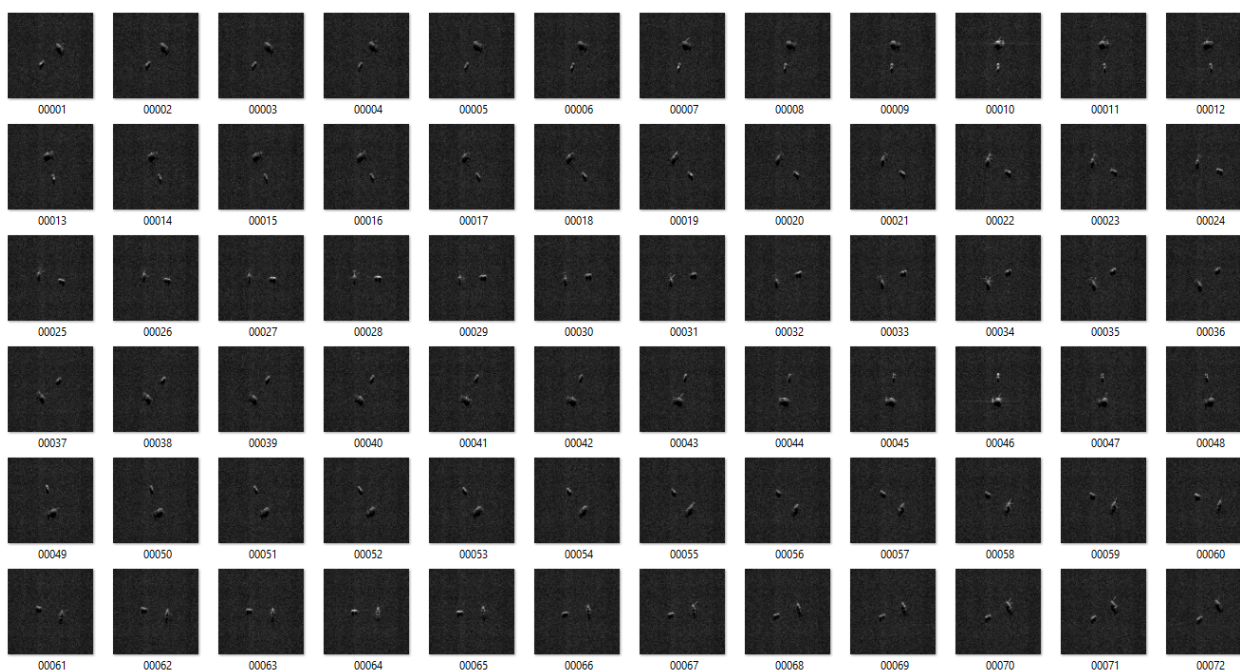
Figure 3-8: SAR images of data augmentation with two targets and multiple azimuth angles to the targets.
