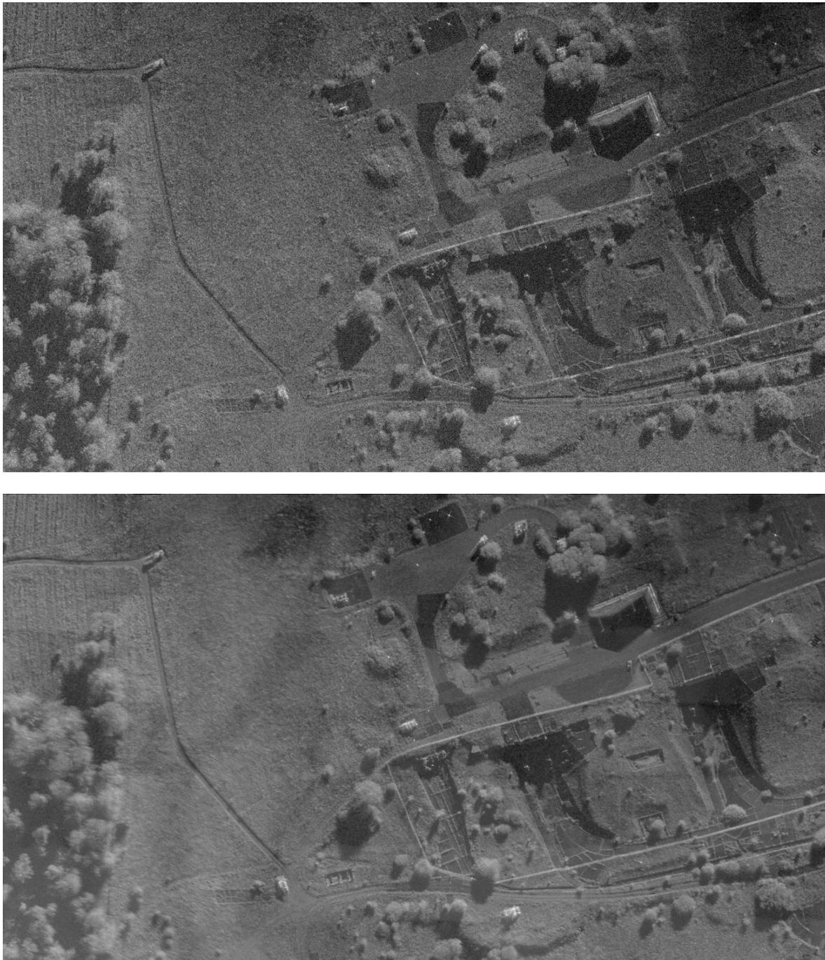
**Figure 6: Comparison of a single look (top) and a multi-look SAR image (bottom). The rectangular mark is referenced in Section 5**
