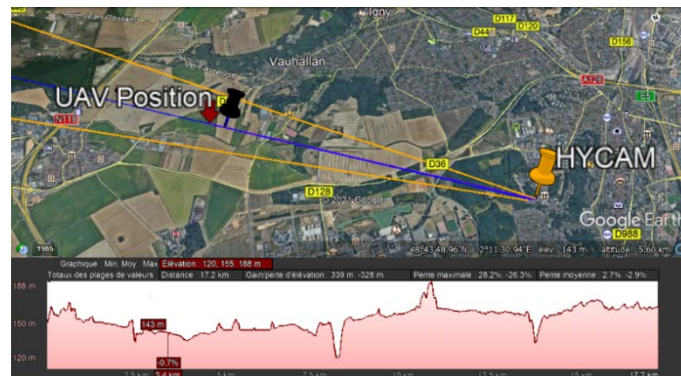
Figure 2 Map with HYCAM position and the UAV position during the measurement. The aiming line is the blue line and the orange lines are the limits of the main lobe.
