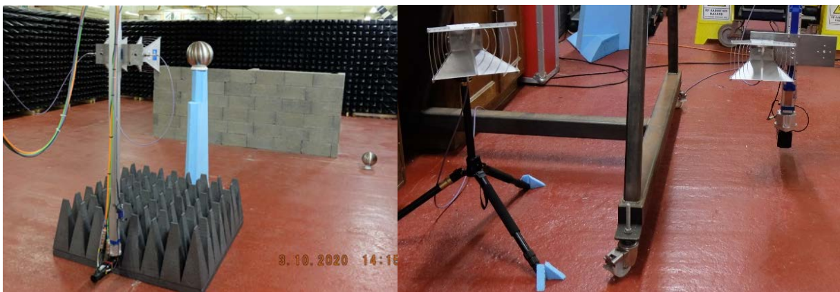
Figure 3 1, Microwave antennas in monostatic configuration undergoing calibration (left), and in bistatic configuration (right).
