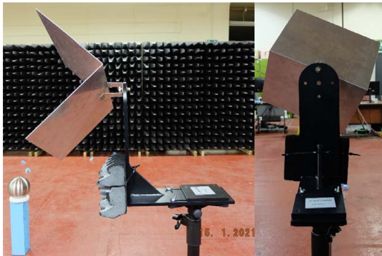
Figure 3-2, Sphere and dihedral targets. The dihedral was rotated to multiple angles.
