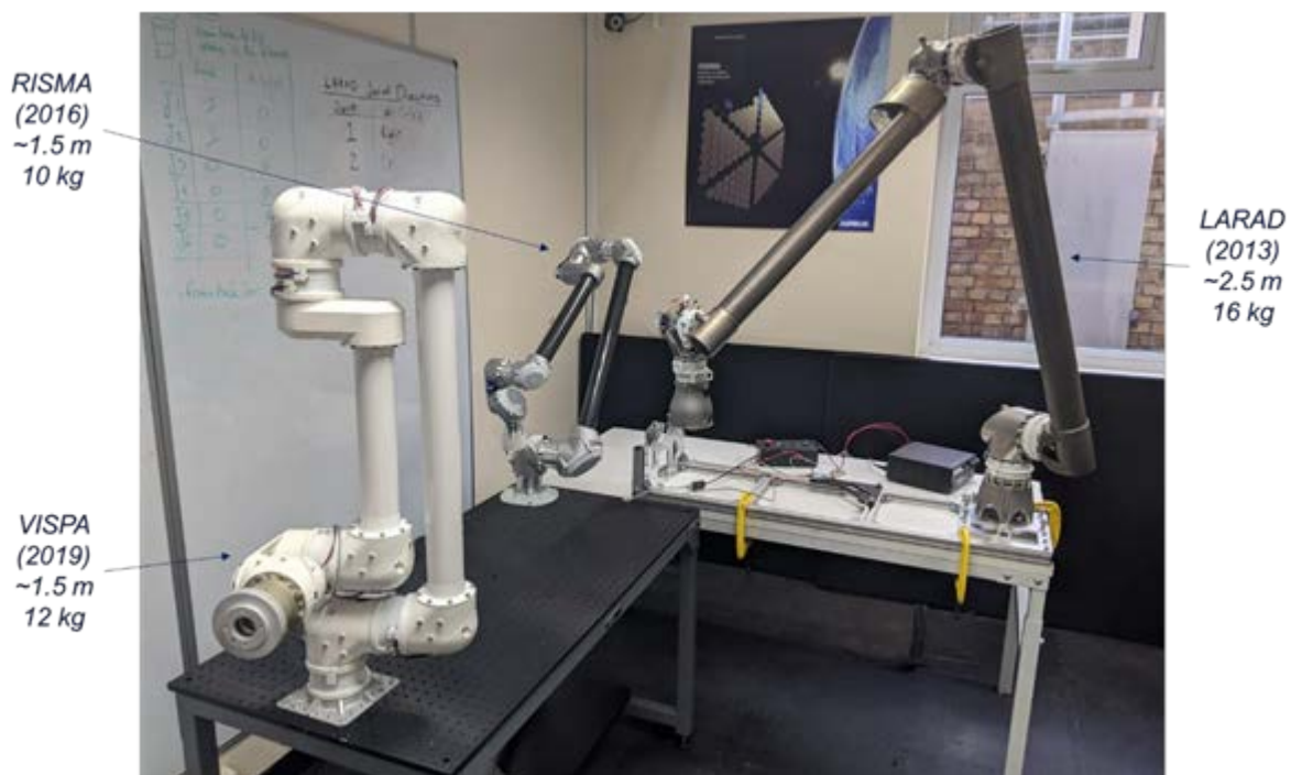
Figure 6: Airbus robotic arms for in-orbit servicing showing the development year, total reach, and mass of each arm (Credit: Airbus)
