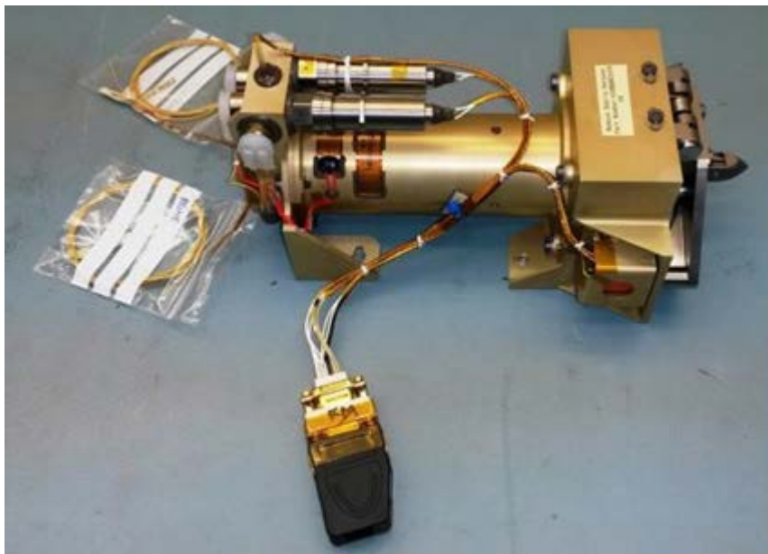
Figure 2: RemoveDEBRIS harpoon prior to installation of multi-layer insulation (Credit: Airbus)
