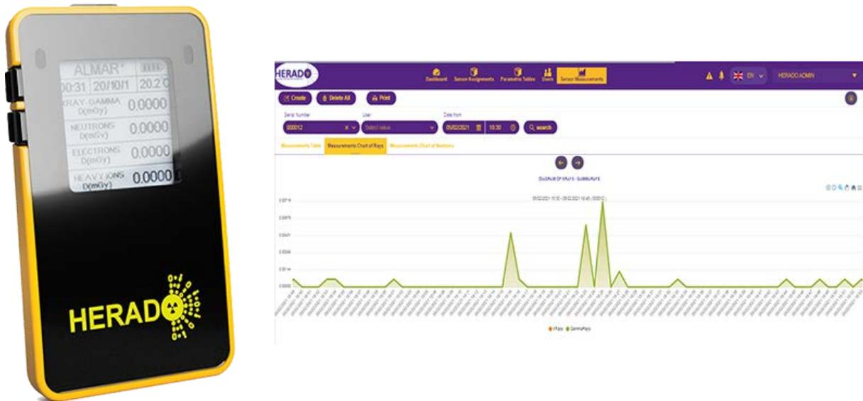
Figure 3: HERADOs, ALMAR dosimeter and software
