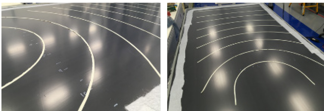
Figure 4: Photographs of the AFP deposited tape after the steering trials.
