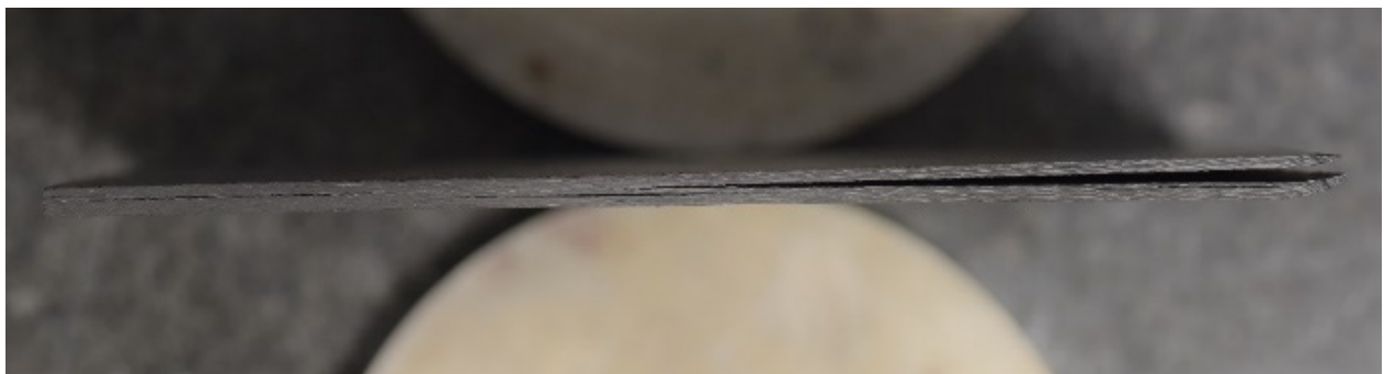
Figure 4: Severe delamination occurred during pyrolysis.
