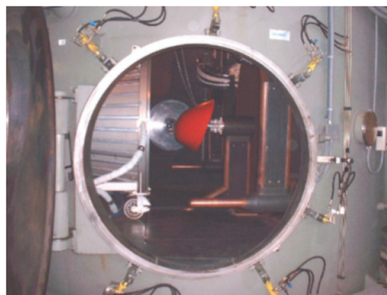
Figure 16: SCIROCCO test chamber.
